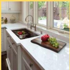
The material itself is an engineered product that's made mostly from ground quartz compressed with different amounts of fillers or resins under intense heat and pressure. The more filler added to the material, the less expensive the quartz countertop gets.
